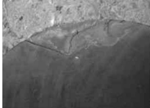
Figure 2 - Crack appearance of macroscopic test piece
