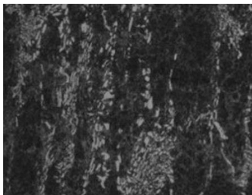
Figure 8 - Non-uniformity of eutectic carbide (100 X)
